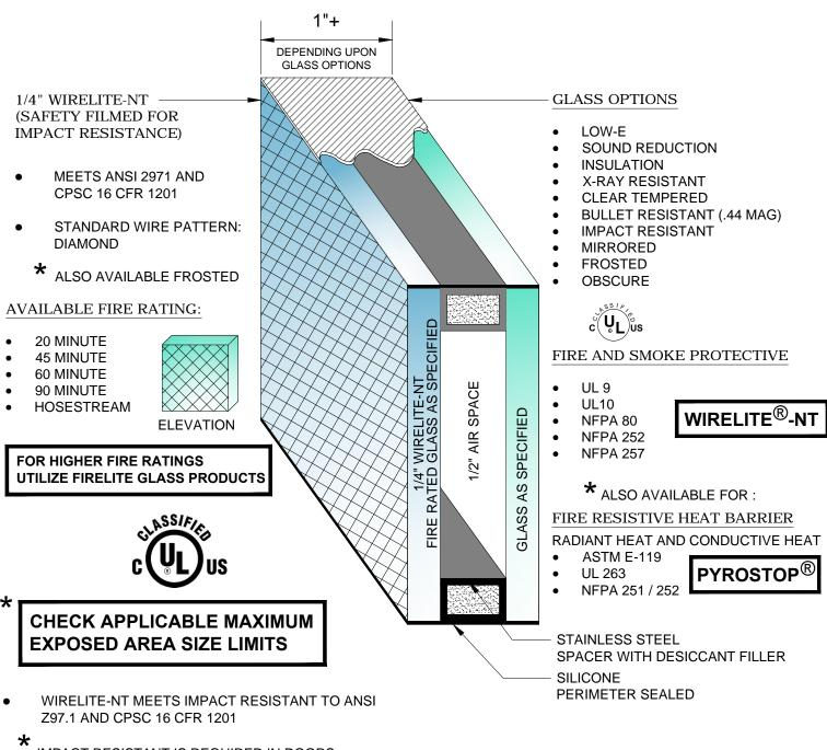
IMPACT RESISTANT IS REQUIRED IN DOORS OR IN WALLS WITHIN 24" OF DOOR OPENING
