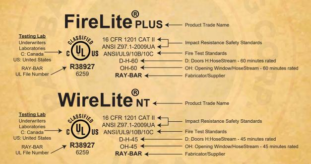
\*Fire Protective: Barrier to Flame and Smoke: \*Fire Resistive: Barrier to Flame,Smoke and Radiant Heat \*(Meets: UL 9, 10B, 10C and NFPA 80, 252, 257) (Additionally meets: ASTM E-119, NFPA 251, UL 263)
