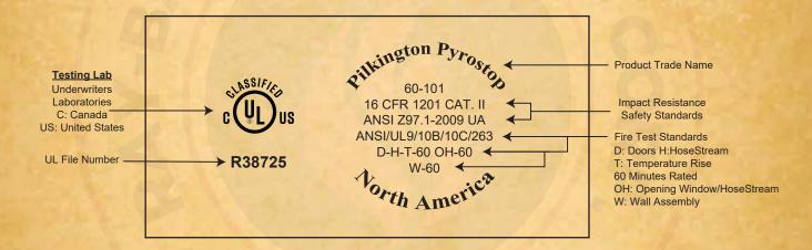
\***Fire Protective**: Barrier to Flame and Smoke\* \***Fire Resistive**: Barrier to Flame,Smoke and Radiant Heat \*(Meets: UL 9, 10B, 10C and NFPA 80, 252, 257) (Additionally meets: ASTM E-119, NFPA 251, UL 263)
