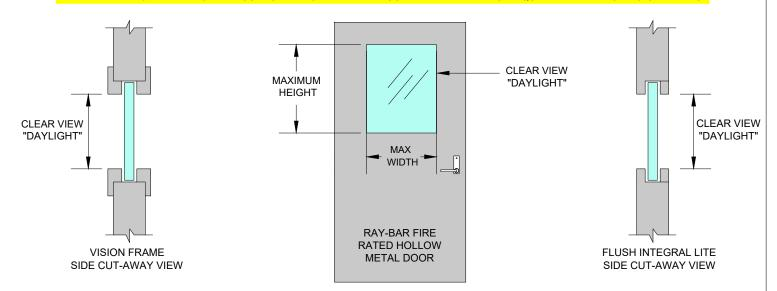
MAXIMUM CLEAR VIEW "DAYLIGHT" GLASS OPENING SIZES PERMITTED FOR FIRE RATED HOLLOW METAL DOORS
